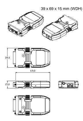
Note: The transmitter, M1-201DA-Tx and the receiver, M1-201DA-Rx have the same mechanical dimensions.
