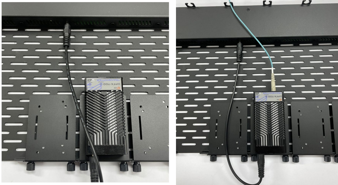
Fig. 10: Mounting the DPFX-700-TR/HDFX-700-TR Module bracket on BR-400.
