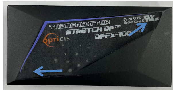
Fig. 11: Remove DPFX-100-TR upper part label and screws
