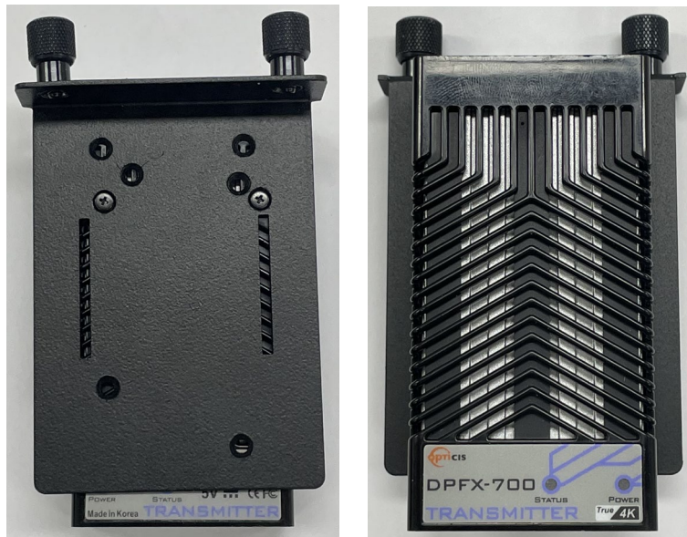
Fig. 8: Mounting screws into bracket holes
